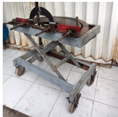
Figure 5. Welding Table Prototype in SMAW Welding Based on Worker Anthropometric Data
